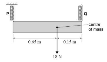
The top end of spring **P** is fixed and the top end of spring **Q** is adjusted until the sign is horizontal and in equilibrium.
