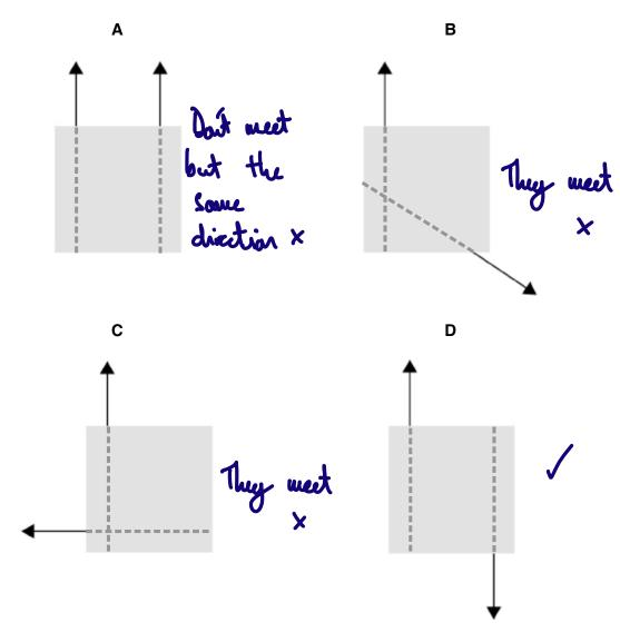
Which system produces a couple about any point inside the object?
